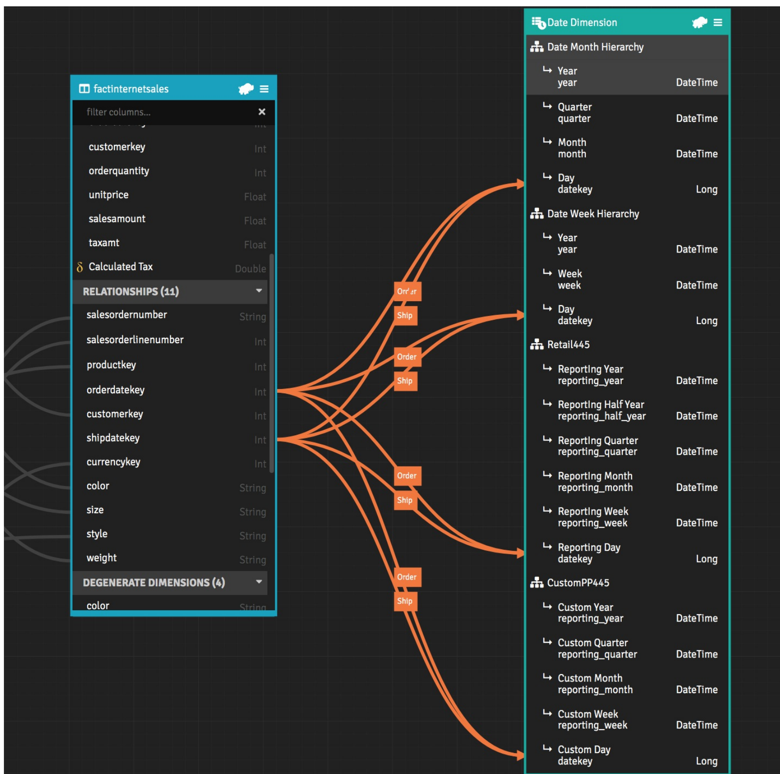
Figure 1. Role-playing relationships: The Date dimension is in relationships to orderdatekey and shipdatekey in a fact dataset. The top four relationships trace to the Month and Week Hierarchies of the Date Dimension.
