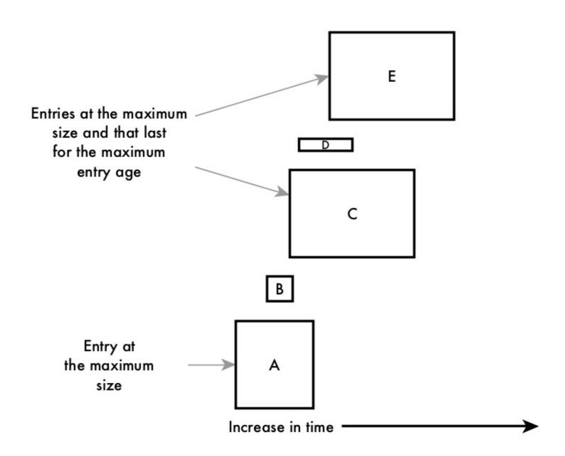
The last diagram shows greatly simplified interactions between entry age, entry size limit, and eviction size limit. The diagram is a chart that shows the total number of cells in the query cache along the vertical axis and arbitrary, equal units of time along the horizontal axis. All rectangles of a single color constitute a single entry. The maximum entry age is set to be five of these units, as shown by entry C.
